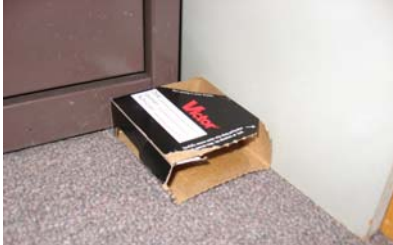
Figure 2. Matchbox monitoring station
